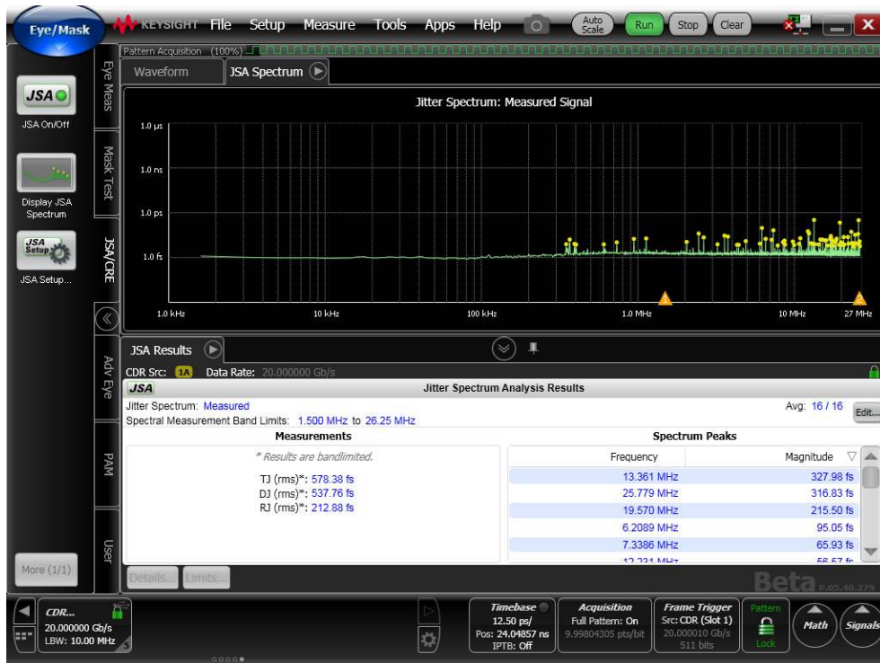
Figure 11. Jitter spectrum analysis (N107xA Option JSA) optimizes Jitter Mode (86100D Option 200) accuracy, measures low-frequency jitter (phase noise), and provides insight into the root cause(s) of jitter.
